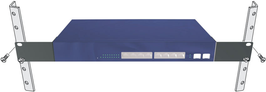
Figure 15: Installing the Switch in a Rack
