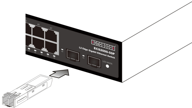
Figure 15: Installing an Optional SFP Transceiver into a Slot
