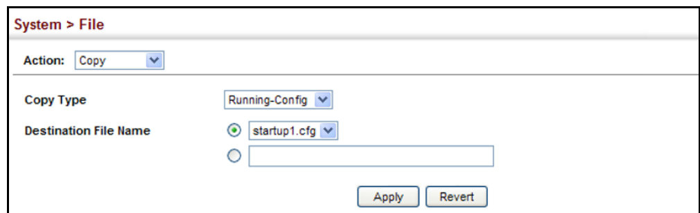
Figure 8: Saving the Running Configuration
