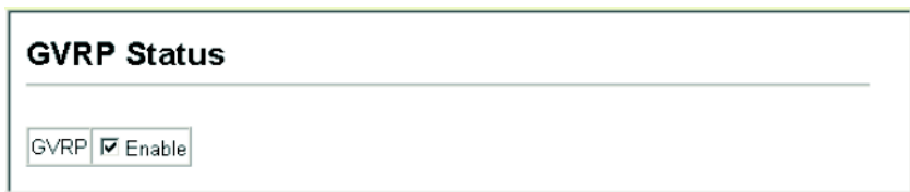
Figure 3-94 Globally Enabling GVRP
