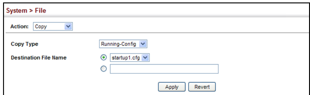
Figure 8: Saving the Running Configuration
