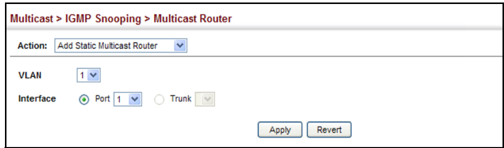
Figure 324: Configuring a Static Interface for a Multicast Router
