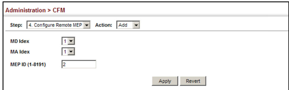
Figure 303: Configuring Remote Maintenance End Points
