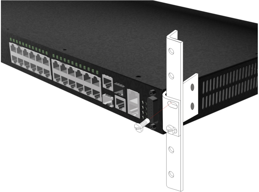
Figure 9: Installing the Switch in a Rack
