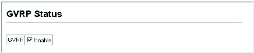
Figure 12-1 Globally Enabling GVRP
